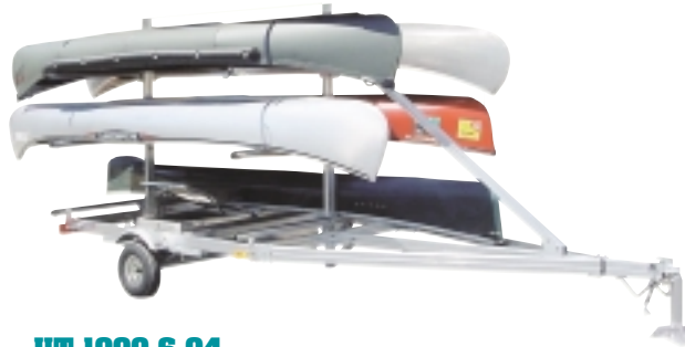
UT-1000-6-04 This all bolted aluminum trailer has a 1000 pound capacity and weighs 305 lbs. It is fully adjustable for carrying 6 canoes up to 18' in length. Standard adjustable crossbars with vinyl extrusions to protect your boats. (Shown with optional storage box)
