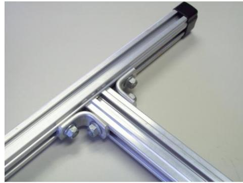
**(Pencil marks.) Install 3 cross bars to the T-bolts in the wide sides of the uprights. Align the center of the cross bars with the pencil marks on the uprights.**
