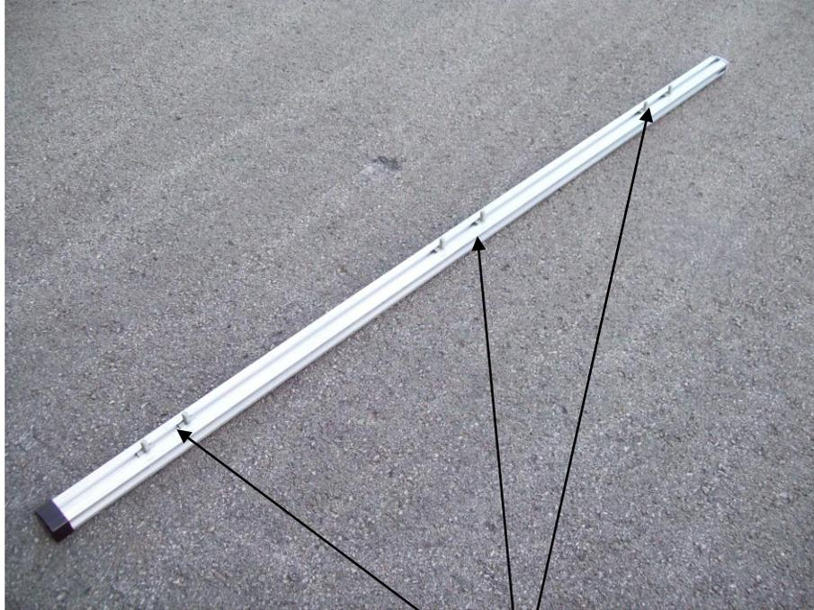
**Lay out the four 66 inch uprights and install 6 T-bolts in the wide side and 4 T-bolts in the narrow side of each. (Pencil marks.)**
